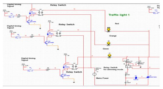
When a digital high signal is received from subsystem 2, the incandescent lamp is turned on and when a low signal is received, the incandescent lamp is switched off as shown in the following respective figures:
