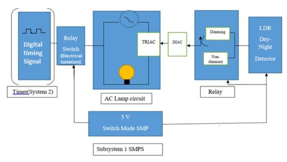
The preceding block diagram will be replicated for each light bulb, with the exception of sharing the same dimming circuitry. A parallel configuration of the incandescent bulbs will be implemented, and any dimming effects caused by this configuration due to current division will be negligible.
