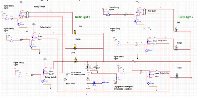
The digital timing signals will be obtained from Subsystem 2 and are represented as 5V signals in this circuit diagram. In the aforementioned figure, the daylight circuit has been simplified and will be substituted with the following circuitry for detecting day and night with hysteresis:
