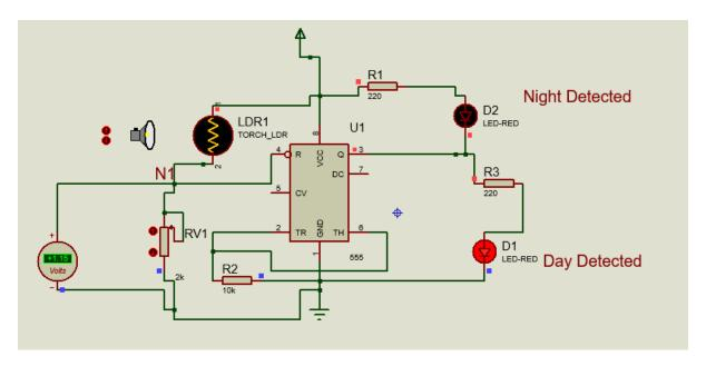
The output detected can then be used to control a relay switch, which will dim the traffic lights, as discussed in the latter section.
