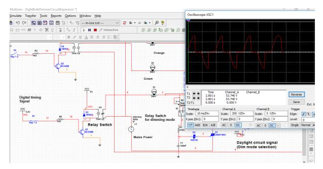
After dimming, by adjusting the potentiometer or initially calibrating it, the following waveform and brightness is visibly shown. Note that the daylight detector switch is closed:
